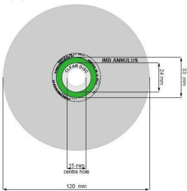
Inner Diameter: 34mm Outer Diameter: 116mm
