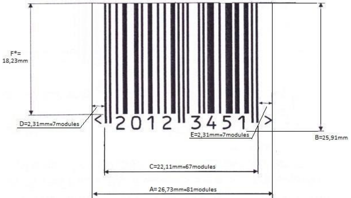
Fig 4. Nominal dimension bar code EAN-8 for the magnification factor 1.0
