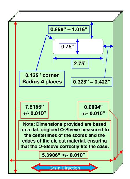
Back Side of O-Sleeve Finished Product Shown for Dimensions Only, refer to Page 1 for proper folding.
